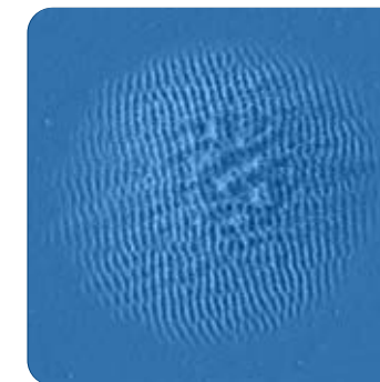
Surface functionalization with conventional system (Gaussian Beam)
