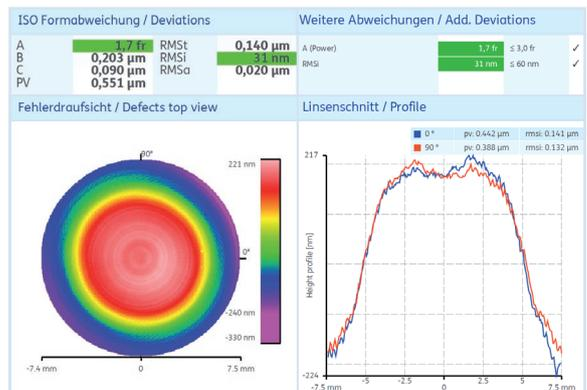
Full surface measurement of surface form deviation of the freeform element, showing the outstanding quality with a RMS<sub>d</sub> of 31 nm.
