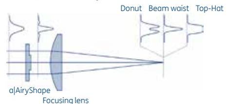
Consisting of phase plate and focusing lens, with correlated intensity distributions in the focal region
