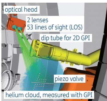
Fig. 1 Injected helium cloud excited by collision with plasma electrons and emitted light to be spectroscopically analyzed
