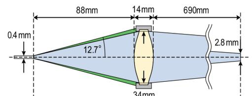
Fig. 3 Schematic representation of optical head
