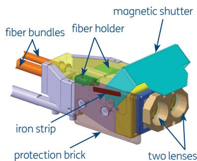
Fig. 2 CAD drawing of the optical head
