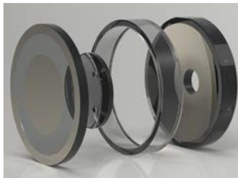
Fig. 2 Manufactured mirror optics and spacer
